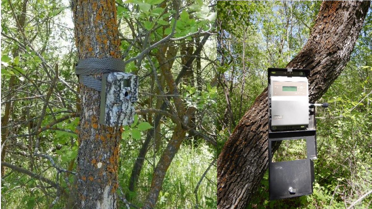
Figure A-III 9. Autonomous recording devices at Maple Grove. LEFT: wildlife camera. RIGHT: acoustic recorder. (Meewasin, 2021).
