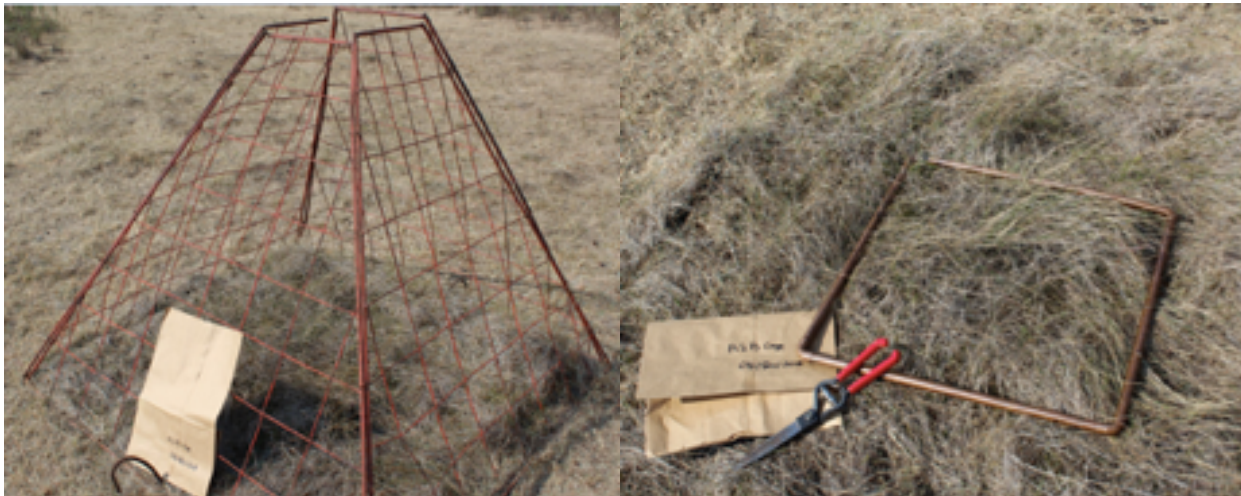
Photo 1d: Grazing exclusion cage and vegetation transect clipping process used to monitor intensity of targeted conservation grazing (Location: Northeast Swale).
