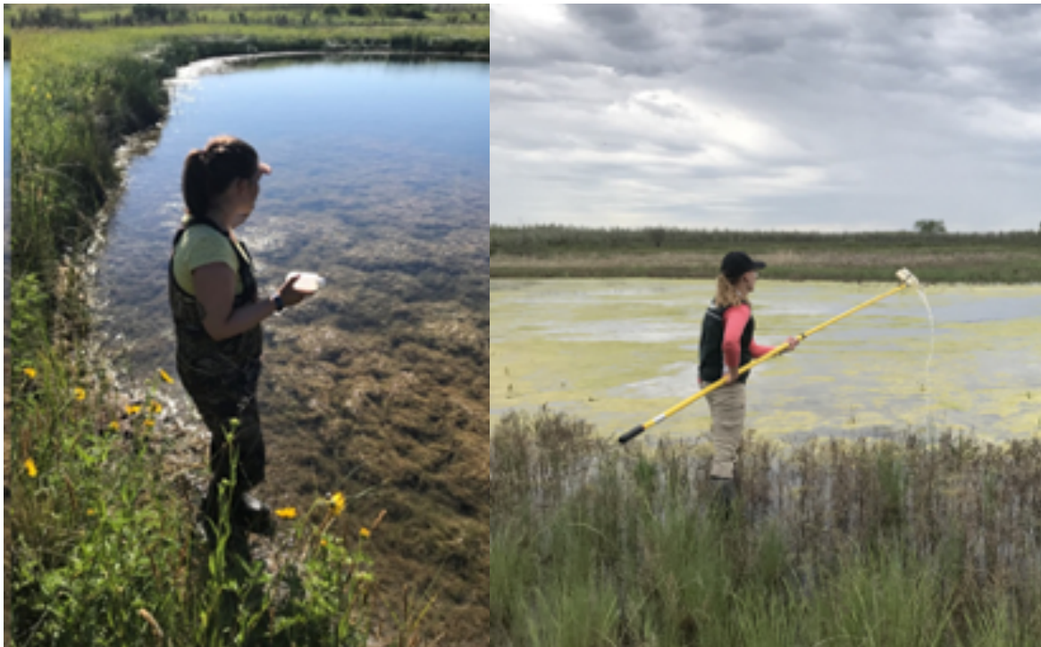
Photo 1f: Collecting grab samples for water quality testing (Location: Small Swale).
