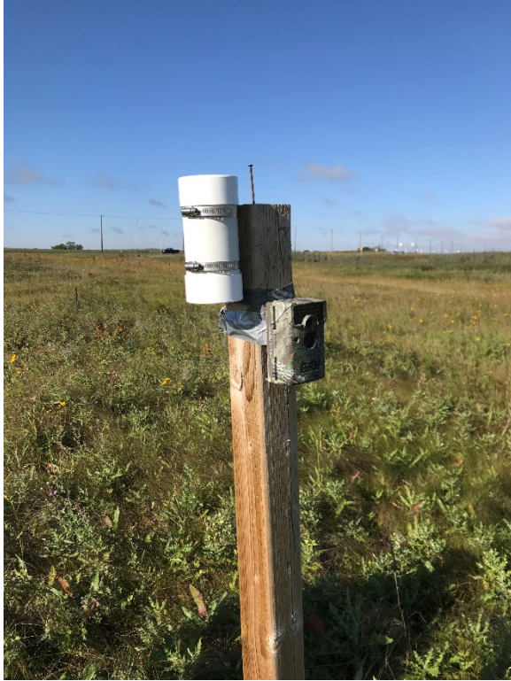
Photo 1a: Meewasin permanent monitoring plot equipped with a SQM-L Dark Sky Meter and Wildlife Camera (Location: Northeast Swale).
